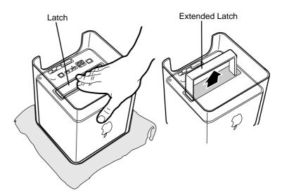
Gently pull the core from the computer enclosure and place the core on a soft cloth.
